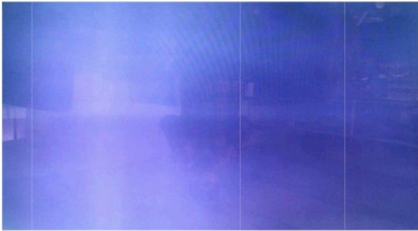
Figure 1. Displayed image of 55-inch OLED Panel before compensation.
